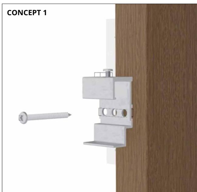
**STEP 4A** Screw WEO Brise Soleil one by one using the clip (FD1154). Use stainless steel self-drilling screw A2 5.5x32mm (FD1155 / FC2628)
