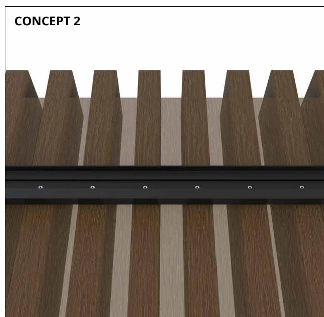
**ÉTAPE 4B** Screw WEO Brise Soleil together as a panel using the FD1156 aluminum rail cut to length. Use stainless steel self-drilling screw A2 5.5x32mm (FD1155).
