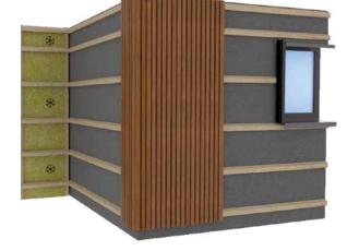
The coating of the composite wood with a polyethylene film over its entire surface ensures protection against any moisture pick-up. It is also not sensitive to stains and discolouration.
