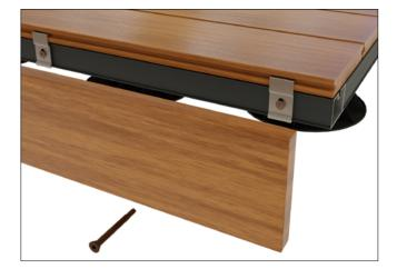
4.2 - Screw the first board. Place the clips in the grooves of the board and also of the joist, by making a simple hand pressure
